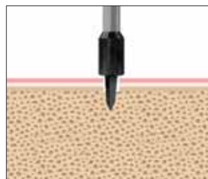
2. Creation of the insertion point with the centring drill
