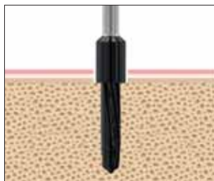
3. Calibration of the final diameter of the implant site with the trimming drill
